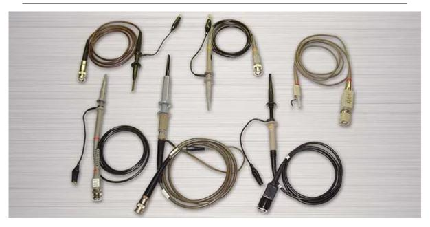
OSCILLOSCOPE PROBES AND PROBING Do you get erratic results with your oscilloscope? Case 3:17-md-02801-JD Document 1063-7 Filed 01/06/20 Page 25 of 39 As you start probing higher and higher frequencies, do the results get increasingly odder? Let's address the reasons for that strange behavior and construct an Active Probe for a low price.
